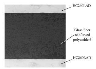
Figure 4. Sectional microscopic microsection of a hybrid laminate after the cathodic dip painting process
